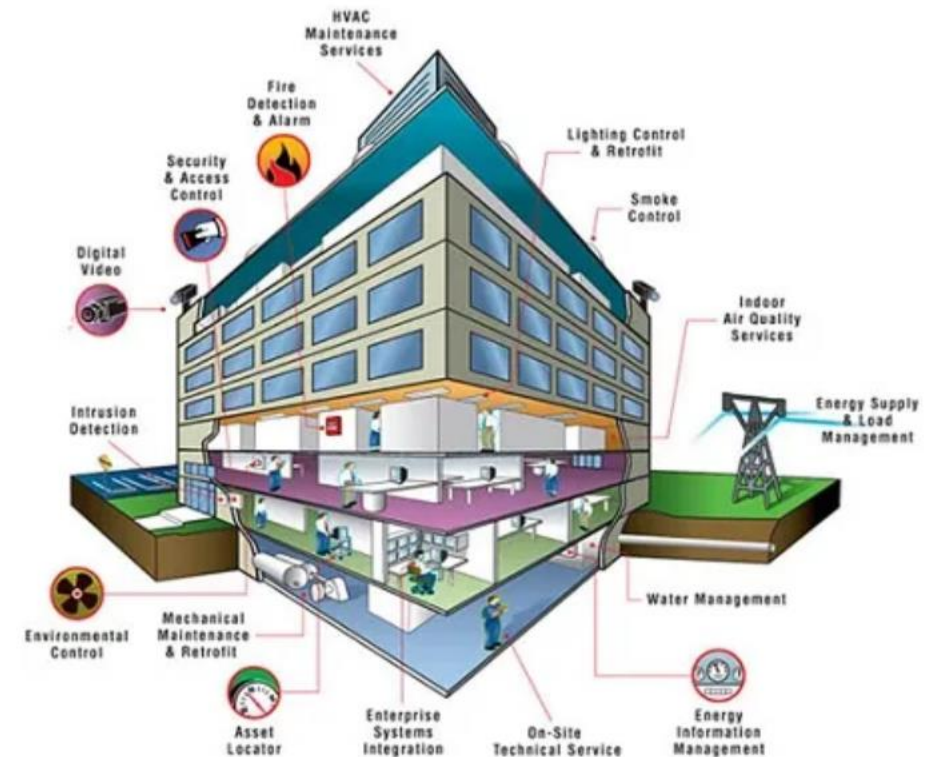
BAS applications in a commercial building
